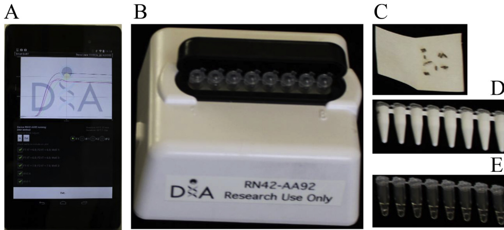
Fig. 1. Smart-DART™ technology for detection of Candidatus Liberibacter in citrus psyllids. A custom app installed on an Android device (A) is used via Bluetooth® to operate the Smart-DART™ (B). The lid of the unit is partially opened to show the 8 reaction tubes inside. Psyllids are air-dried at 25 °C for 2–5 min (C) and dropped into extraction tubes (D) and incubated in Smart-DART™ at 85 °C for 10 min to extract crude DNA. 5 µL of the extract is transferred to reaction tubes (E) and the LAMP reaction is carried out in Smart-DART™ at 65 °C for 20 min. Amplification graphs are visualized on the Android device which records the data as comma delimited values which can be shared by e-mail or viewed later within the app.
